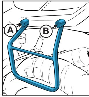
EN\_Remove the original screws supporting the handle on the side where the frame will be mounted.
