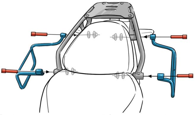
**EN** EN Whenassemblingtheframe, it is important to tighten the screws only onceallparts are assembled. Start by inserting the screws without tightening.
