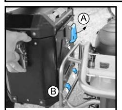
EN: Make sure the mechanism (A) is in the open position. Hook the case to the frame in (A) and (B).
